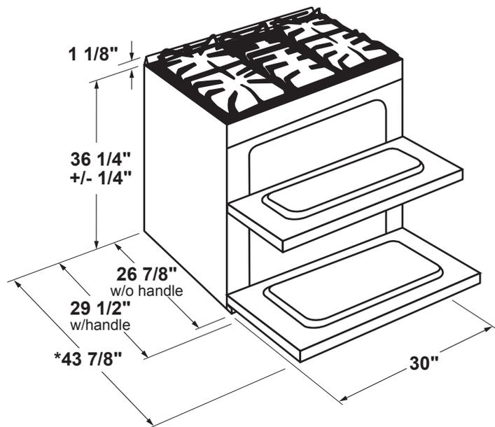
\*Dimensions are referenced from the point at the back of the range that will contact the rear wall first.
