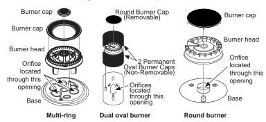
B. Using a 7 mm or 9/32" nut driver, remove the top burner orifices. These may be accessed through the burner opening in the base.
