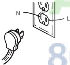
Insure proper ground and firm connection before use
