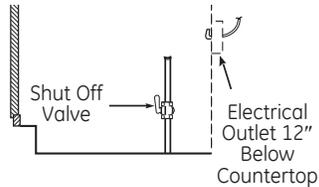
Install a manual shut-off valve in the gas line in an easily accessible location outside the cooktop. Be sure you know how and where to shut off the gas supply to the cooktop. Install the electrical outlet 12" below the countertop.
