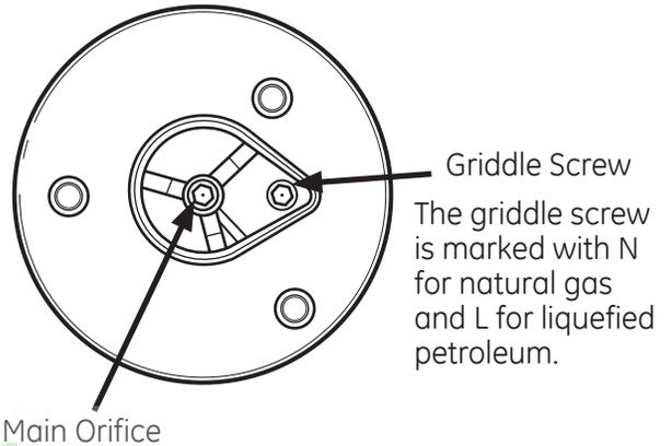
**NOTE:** The main orifice is located in the center of the burner, while the griddle screw is located to the right of the center of the burner.
