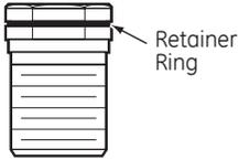
**NOTE:** On all burners, the orifices have a spring-loaded retaining ring around the hex head to hold the orifice in the nut driver during installation and removal. A slight amount of force is required to push the nut driver down over the ring.
