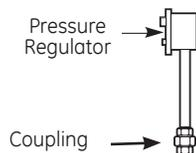
To reduce the likelihood of gas leaks, apply teflon tape or a thread compound approved for use with LP or Natural gases to all threaded connections.
