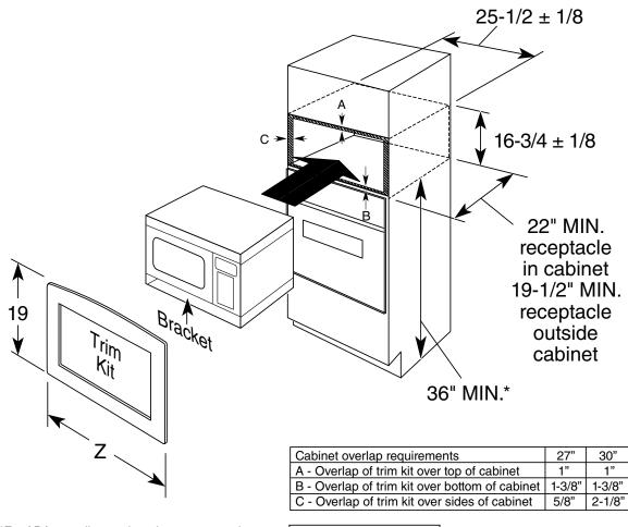
\*For ADA compliance, the microwave must be installed no higher than 36-1/4".
