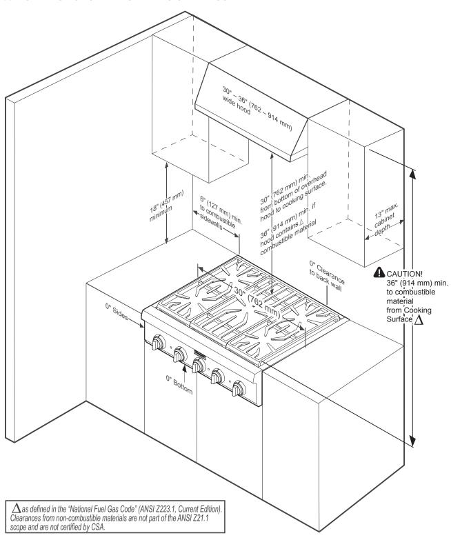
**NOTE:** A 36-inch minimum clearance is required between the top of the cooking surface and the bottom of an unprotected cabinet. A 30-inch clearance can be used when the bottom of the wood or metal cabinet is protected by not less than 1/4 inch of a flame retardant material covered with not less than No. 28 MSG sheet steel, 0.015 inch (0.4 mm) thick stainless steel, 0.024 inch (0.6 mm) aluminum, or 0.020 inch (0.5 mm) thick copper.
