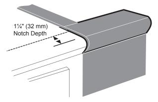
Front flush with cabinets; minimum of 24<sup>9</sup>/16<sup>"</sup> (624 mm) cabinet depth required.
