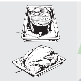
The temperature probe has a skewer-like probe at one end and a plug at the other end that goes into the outlet in the oven.
