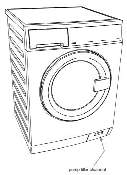
Pump Cleanout/Manual Drain
