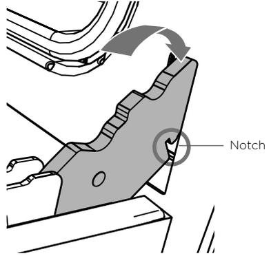
① Hold the door firmly in an approximately halfway open position.
