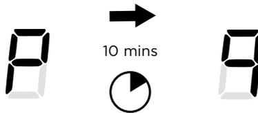
The cooking zone will remain on PowerBoost for a maximum of 10 minutes. After 10 minutes the cooking zone will automatically reduce its heat to setting 9.
