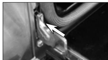
Fig. 08 Hinge retainer clip in locked position
