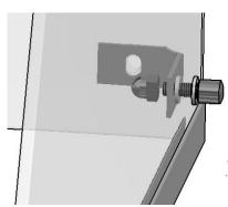
Prepare one set of fasteners for each assembly position
