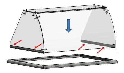
Place the sneeze guard on the freezer, press the sides to the inner side of the box, and fasten the sides to the freezer Look at the picture
