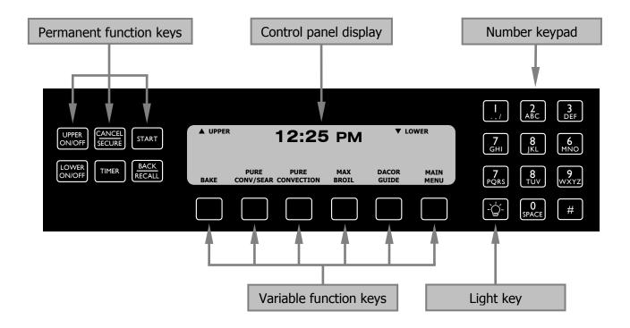
**NOTE:** If you have a *single oven*, you **cannot** set the clock, temperature scale, display colors, keypad tones, or disable the oven lights while the oven is in use. If you have a *double oven*, it is best not to change these settings while the oven is in use.
