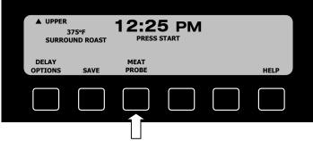
• You will see the preset meat probe temperature of 170°F appear on the display. Consult the <u>Internal Cooking Temperatures</u> chart on page 48 to see the recommended meat probe temperatures for a variety of foods. If the correct meat probe temperature already appears on the display, press **START**. Otherwise, enter the correct meat probe temperature on the number keypad (for examples press **1** than **6** than **9** for **1**(0°F) than
