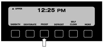
You will see the preset temperature of 100°F appear on the display. To proof at that temperature, simply press **START**. If you want to proof at a different temperature, enter the temperature on the number keypad (for example: to proof at 120°F, press **1**, then **2**, then **0**), then press **START**.
