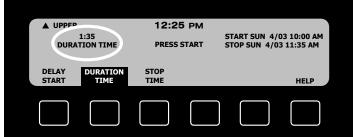
• If you did not enter a start time, the oven will start immediately and stop after the amount of duration time entered has elapsed. If you entered a start time **"WAITING TO START"** will appear on the display. The oven will turn on at the start time that was entered and stop cooking after the amount of duration time entered has elapsed.
