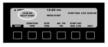
**NOTE:** You may press **START** after you set up the start time and start day without setting the stop time or duration time. If you do so, the oven will start at the specified time and continue to run until you turn it off.
