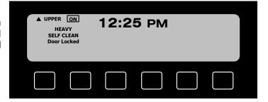
**IMPORTANT:** If you do not shut the oven door completely, the automatic door latch will not lock. The phrase "CLOSE OVEN DOOR" will flash on the display if the door is ajar. To correct the problem, press the CANCEL/SECURE key twice and wait approximately 1 minute. When the door is properly closed, start the self-clean process again.
