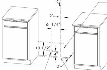
Shortest connection from hard pipe stub location to range hook-up
