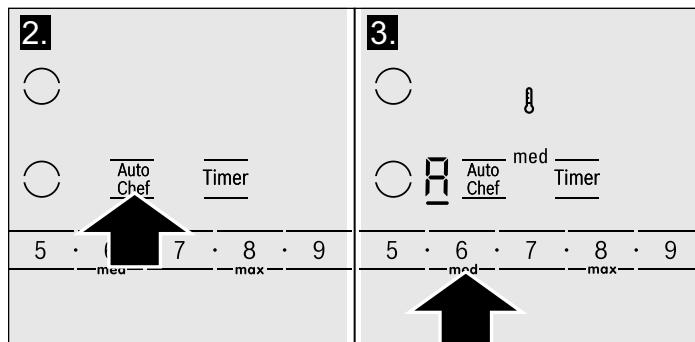
The temperature symbol **flame** stays lit until the temperature is reached. Then a beep sounds, **flame** disappears.
