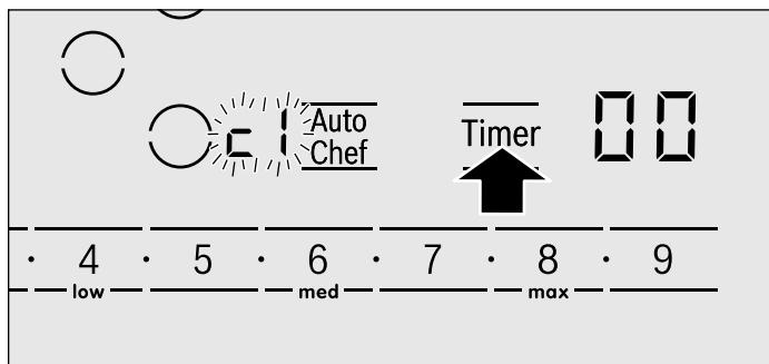
3. Touch **Timer** repeatedly until the indicator for the desired function appears in the element display.
