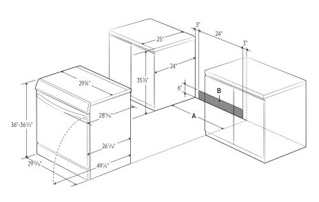
A: Cabinet opening min 30" B: Acceptable electrical outlet area
