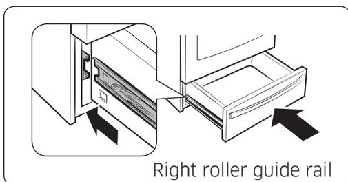
1. Position the ends of the full-extension roller guide rails in the side rails of the drawer opening.
