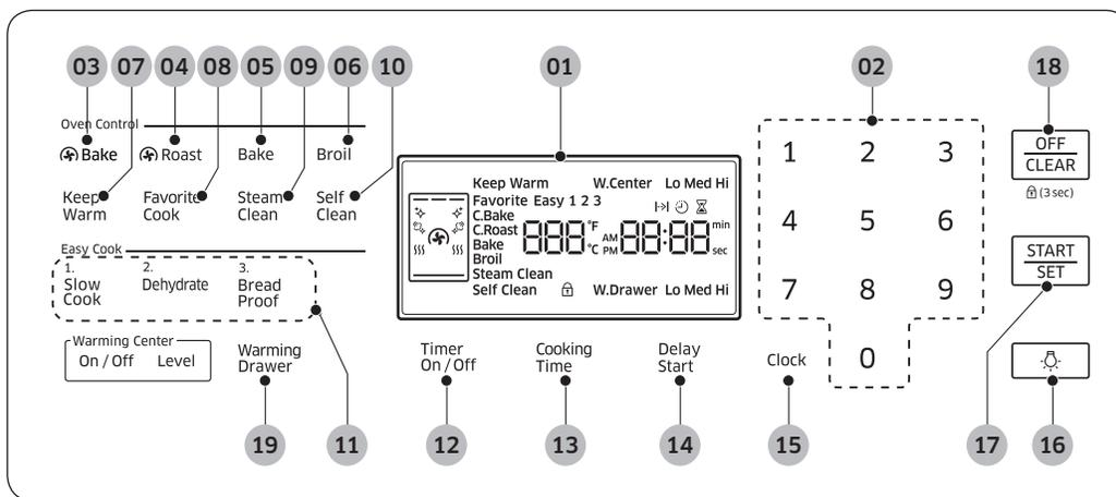
**01 DISPLAY:** Shows the time of day, oven temperature, whether the oven is in the bake, broil or self-cleaning mode, and the time set for the timer or automatic oven operations.
