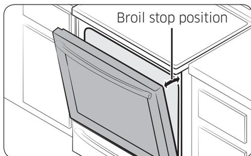
Leave the door open at the broil stop position. The door will stay open by itself, yet the proper temperature is maintained in the oven.
