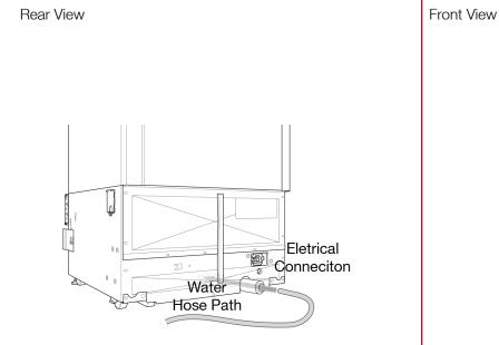
Electrical - 5 foot (1.52 m) - 120 Volt - 15 Amp - NEMA 5-15 molded plug Water line - 1/4" flexible water line - not included Water connection is located in front of unit. 1/4" compression fitting is needed.
