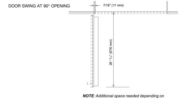
thickness of front panels and handle used When installing hinge side next to an appliance or object that is within range of the door panel, limit the door opening angle to 90°. This is done by installing the banking pin as illustrated. Insert the banking pin through the holes and drive in with a hammer.
