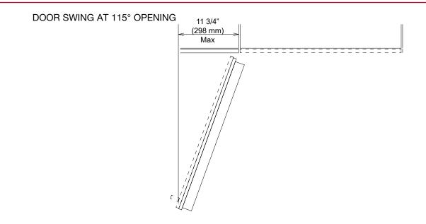
**NOTE**: Additional space needed depending on thickness of front panels and handle used
