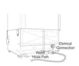
Electrical - 5 foot (1.52 m) - 120 Volt - 15 Amp - NEMA 5-15 molded plug Water line - 1/4" flexible water line - not included Water connection is located in front of unit. 1/4" compression fitting is needed.
