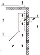
Regulations concerning the discharge of air have to be fulfilled. 6.Install wall cap or roof cap. Connect round metal ductwork to cap and work back towards the hood location. Use duct tape to seal the joints between duct work sections.
