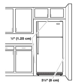
To ensure proper ventilation for your refrigerator, allow for  $^{1}/_{2}$ " (1.25 cm) space on each side and at the top. Allow at least 2" (5.08 cm) between back of cabinet and the wall. If your refrigerator has an ice maker, make sure you leave some extra space at the back for the water line connections.
