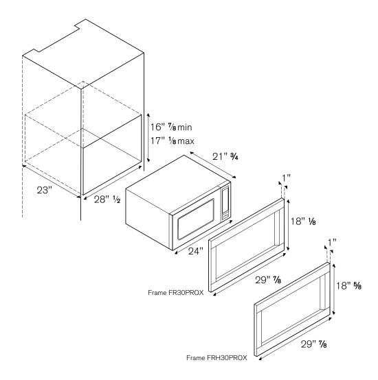
The minimum gap between the kichen cabinet upper or lower panel and the appliance is 1/8. This dimension must be added to the height listed in the drawings
