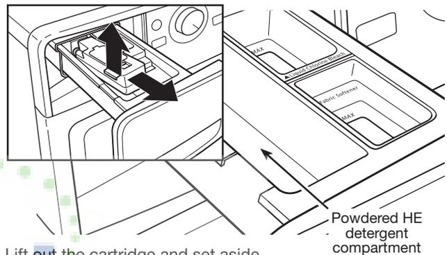
Lift out the cartridge and set aside.
