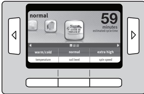
To adjust settings, use the selection button beneath the desired option. If the screen shows the multiple page symbol
