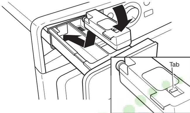
Use only HE High Efficiency liquid detergents. The dispenser cartridge will hold about 18.5 oz. (550 ml) of HE liquid detergent, or enough for up to 36 loads<sup>†</sup>.
