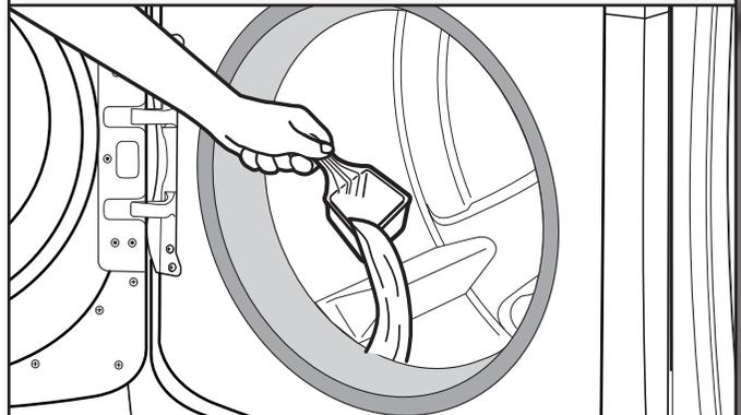
Oxi-type boosters or color-safe bleach can be added to the drum prior to adding laundry.
