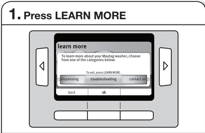
With the washer on, press LEARN MORE to access the built-in troubleshooting feature. Use the LCD control buttons to select TROUBLESHOOTING.
