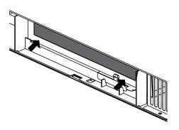
6 Reinstall the vent by sliding the bottom of the vent into place. Push the vent top into position and slide right into place. Replace the two vent mounting screws located on top of the microwave using a #1 Phillips screwdriver.
