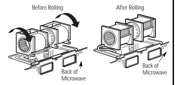
Remove the knockout plates in the back of the unit with snips. (For some models) Knockout Plates:
