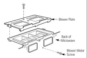
Remove the screw that holds the blower plate to the microwave. Remove and save the screw holding the blower motor to the microwave. 2 Carefully pull out the blower unit. The wires will extend far enough to allow you to adjust the blower unit.
