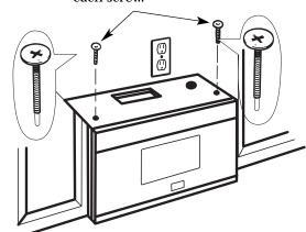
6 Tighten the outer two screws to the top of the microwave oven. (While tightening screws, hold the microwave oven in place against the wall and the top cabinet.)
