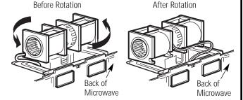
5 Gently remove the wires from the grooves.
