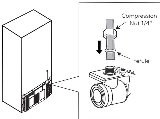
Hold on to the pipe from the handles or grabbers located behind the refrigerator, loosening first the bolt holding the handle. Afterwards, insert pipe into the hole and tighten bolt to finalize.
