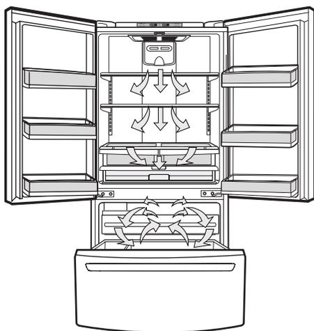
**Do not** block any of these vents with packages of food. This can interrupt the flow of air and cause temperature and moisture problems.
