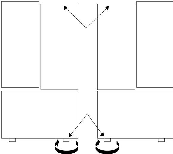
4. Open both doors again and check to make sure that they close easily. If not, slightly tilt the refrigerator further back by turning both leveling screws clockwise. It may take several more turns. Make sure that you turn both leveling screws the same amount.
