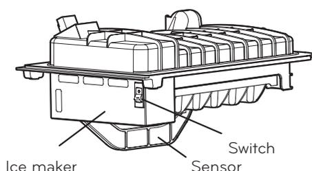
The ice maker produces 12 cubes per cycle (in between 80 and 100 cubes in a 24 hour period), depending on the temperature of the freezer, the times in which the door opens, and other using conditions (amount of food in the freezer, etc).
