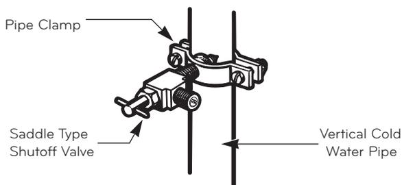
**NOTE:** Codes for 248 CMR pipelines of the state of Massachusetts must be attached to the connection. Valves of this type are banned in Massachusetts. Call an authorized plumber.
