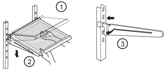
**NOTE:** Make sure that the shelf is installed in the horizontal manner. If not secured it can cause the shelves to fall, which will cause your stored food to spill.
