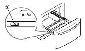
With both hands, grasp the sides of the door and pull it up to separate it from the rails.
