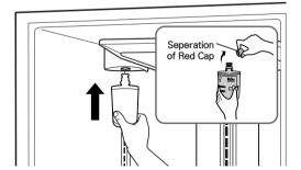
2 Remove the old cartridge. Take the new cartridge out of
