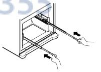
With both hands, hold each rail and push it in to allow both rails to slide in simultaneously.
