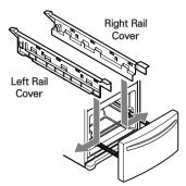
Align the tabs on the covers with the assembly holes on each rail, and snap the rail covers in place to secure.
