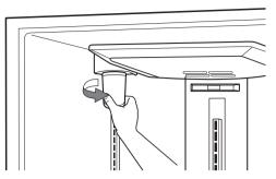
After replacing the filter, flush 2.5 gallons through filter before use (flush for approximately 5 minutes). Check the filter for leaks.
