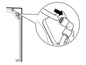
9 Insert the water supply tube at least 5/8 in.(15 mm) into the connector.
