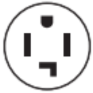
4-wire receptacle (14-30R)
