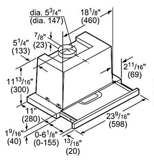
Installation height above cooking surface: 24"-34" (610-864) to Electric 29<sup>1</sup>/<sub>2</sub>"-34" (750-864) to Gas.
