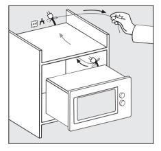
■ Slide the microwave oven into the cabinet space, and pull the cable with the plug through the rear wall of the cabinet.
