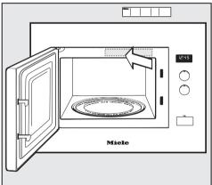
Place the enclosed quick guide to the frame behind the door (as illustrated), making sure they do not block any of the vents.
