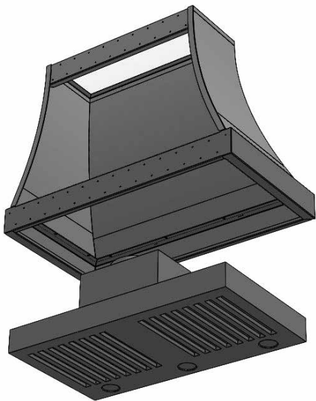
Rear view showing liner is easily removed and reinstalled for simply mounting of hood shell to the wall
