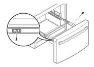
5 Grip both sides of the freezer door and pull it up to remove it from the rails.
