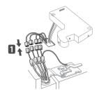
Make sure that the door-switch located inside the cover is tightly connected. Position the cover in place. Insert and tighten the cover screw 2.
