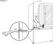
The right refrigerator door does not have an adjustable nut.
