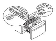
Remove the Durabase™ basket from the rails. Remove the screws from the rails at both ends.
