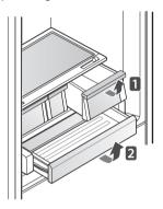
To install, slightly tilt up the front, insert the drawer into the frame and push it back into place.
