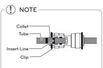
Gently press the collet and insert the tube until only one line shows on the tube.
