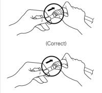
Pull the tube to make sure that the tube is tightly fastened and then insert the clip.
