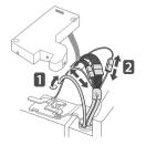
Rotate the hinge lever counterclockwise 1. Lift the top hinge 2 free of the hinge lever latch.
