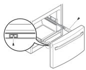
4 Insert the upper pullout drawer into the frame, and push the drawer back into place until you hear a click.
