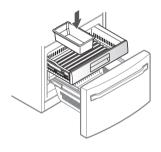
6 Insert the lower pullout drawer into the rail assembly.
