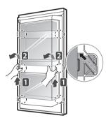
2 To replace the Door-in-Door case, align the tabs on the Door-in-Door case with the slots on the door and push down until it snaps into place.
