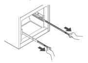
2 Grasp the freezer door on each side and hook the door supports into the rail tabs located on both sides.
