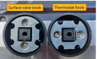
(Incorrect knob caused broken thermostat shaft)
