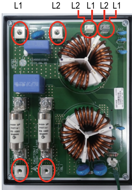
L1 L2 < Noise Filter wiring Check Point >
