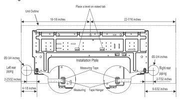
Figure 5: Installation Plate Attaching Screw Placement.
