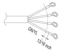
Figure 50: Close up of a Typical Ring Terminal
