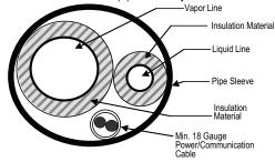
Figure 33: Underground Refrigerant Piping.
