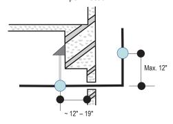
Figure 23: Pipe Support at Y-branch Fitting.
