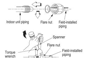
Figure 42: Indoor Unit to Field-Installed Piping Connection.
