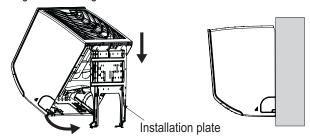
Figure 8: Accessing the Back of the Indoor Unit.
