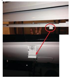
Figure 55: Remove Screws from Bottom Panel
