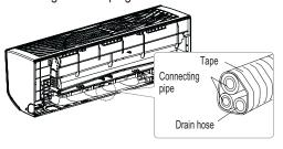
Figure 12: Piping Installed to the Right.
