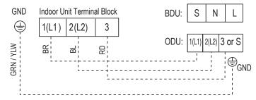
Figure 61: Indoor Unit to Outdoor Unit / Branch Distribution Unit Terminal Connections—LSN180HSV4 and LMN248HVT.
