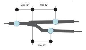
Figure 22: Pipe Support at Indoor Unit.
