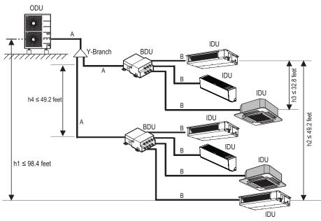
Table 8: Multi F MAX Outdoor Unit Refrigerant Piping System Limitations.
