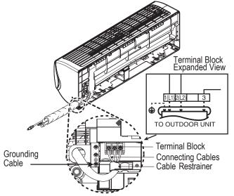
Figure 60: Indoor Unit to Outdoor Unit / Branch Distribution Unit Terminal Connections—LMN078HVT, LSN090HSV4, LSN120HSV4, and LMN158HVT.
