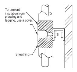
Figure 28: O-Ring Band Support with an Insulated Pipe.
