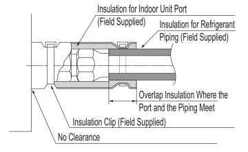
Figure 45: Insulating the Piping.
