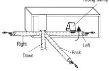
Figure 11: Piping Installed to the Left.
