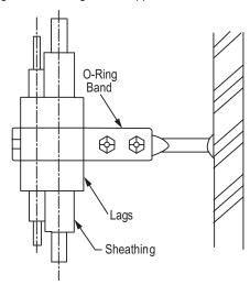
Figure 29: One-Point Down-Stop Support (>441 lbs.).
