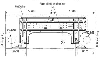
Figure 4: Installation Plate for LSN180HSV4 and LMN248HVT Units.
