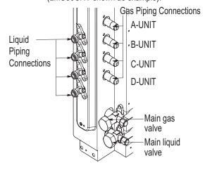
Figure 37: Connection Socket Diagram.
