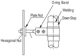
Figure 30: Two-Point Down-Stop Support.
