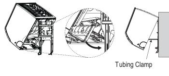
Figure 9: Removing the Frame Cover.
