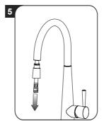
You can now totally remove the hose from the faucet body and replace it with a new hose. Reassemble the hand shower assembly by following the instructions in reverse order:
