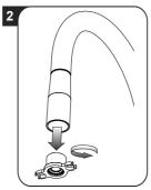
Before removing the aerator make sure that the faucet is turned off. Unscrew the aerator using the aerator installtion key (E) included with the faucet. If the aerator is clogged just rinse it with running water. Do not use detergents. Reassemble the aerator by following the instructions in reverse order.
