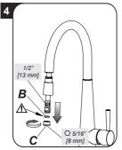
Unscrew the bushing connected to the end of the hose (B) paying attention not to loose the rubber gasket (C).
