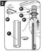
For countertop thicknesses less than 1/16" thick use the rubber gasket (B1) and mounting flange (B2), for all other installations use the rubber gasket (B1) and metal washer (B3).
