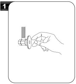
Shut off water supply at angle stop. Clean sink surface in preparation for new faucet.
