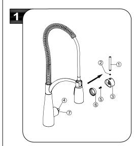
Shut off water supply. With valves in "closed" position. Remove handle (1), loosen the set screw (2). Remove handle seat (3) from valve stem (4). Loosen the screw (5) from valve stem (4) and unscrew the cap (6) from the cartridge nut (7).
