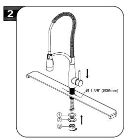
Insert supply hose assembly through hole of sink. From underneath sink, secure faucet with plastic washer (1), metal washer (2) and nut (3). Firmly tighten retaining nut. Do not overtighten.
