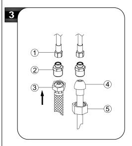
Make connections to water lines with 3/8" female compression supply hoses (1). If additional hose length is needed, attach included 1/2" MIP thread adaptors (2) to supply hoses (1). Use 1/2" I.P.S. faucet connections (3) or use coupling nuts (5) with 3/8" O.D.ball-nose riser (4) to make connections to water lines. Use wrenches to tighten connections. Do not overtighten.
