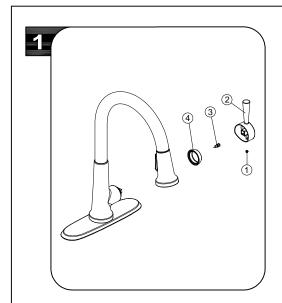
Shut off water supply. Unscrew the set screw (1) on the handle (2). Remove handle (2) and unsrew the screw (3). And then remove cap (4).
