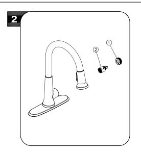
Loosen cartridge nut (1) by turning it counter-clockwise and lift out the cartridge (2). Insert new cartridge. Reinstall the handle.
