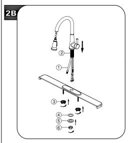
Retract pull-out hose (1) up through faucet body, until the pull-out hose fitting is flush with the bottom of shank (2). Do not pull hose fitting past the shank. Insert faucet body through the hole in escutcheon.
