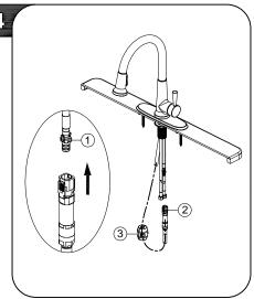
Screw quick connect assembly to the free end of pull-out hose. Align male fitting (1) and tabs (2) on quick connector. Push quick connector housing firmly upward and snap onto receiving male fitting. Pull down moderately to ensure connection has been made.
