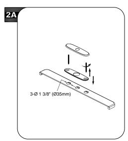
Before installation, screw bolts to the large escutcheon. Insert escutcheon assembly through the gasket and the holes of the sink.
