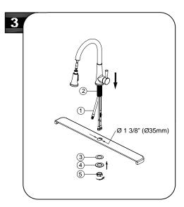
Retract pull-out hose (1) up through faucet body, until the pull-out hose fitting is flush with the bottom of shank (2). Do not pull hose fitting past the shank. Insert faucet body through the hole.
