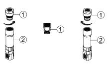
This faucet ships with a 1.5 GPM flow restrictor installed. An optional 2.2 GPM flow restrictor is also included in the box.
