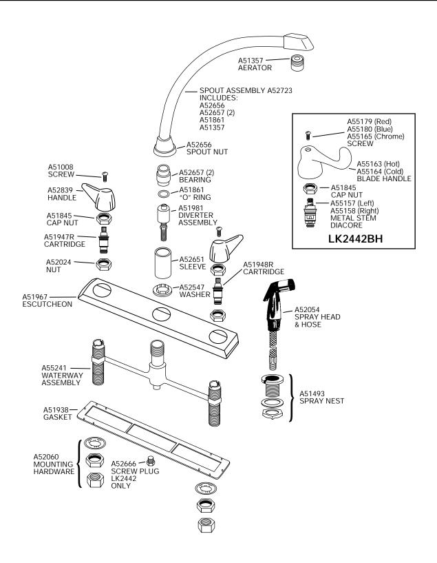
Warning: Blade handles must only be used with A55157 and A55158 Metal Stem Diacore Cartridges.
