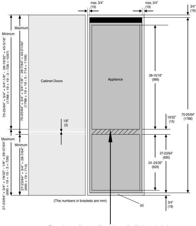
The gap between refrigerator and freezer door must lie within the crosshatched area.
