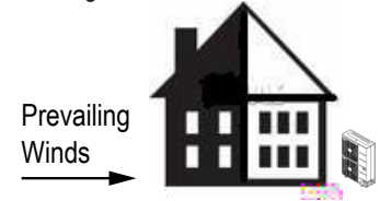
Figure 24: Leeward Side of the Building.
