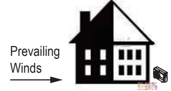
Figure 18: Leeward Side of the Building.
