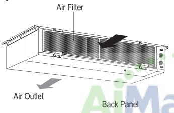
Figure 118: Air inlet from the bottom of the indoor unit.
