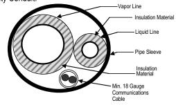
Figure 259: Underground Refrigerant Piping.
