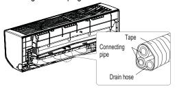
Figure 90: Piping Installed to the Right.
