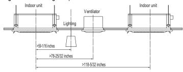
Figure 180: Ceiling Opening Dimensions and Bolt Locations.
