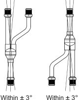
Figure 240: Y-branch Insulation Detail.
