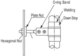
Figure 256: Two-Point Down-Stop Support.
