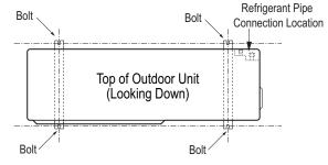
Figure 234: Close up of Bolt Attachment.
