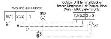
Figure 220: Connecting the Power Wiring and Communications Cable.
