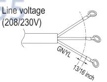
Figure 280: Power Wiring and Communications Cable from the Multi F ODU to the IDUs, or from the Multi F MAX ODU to the BDUs and from the BD Unit to the IDUs.
