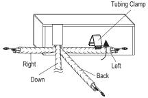
Figure 21: Piping Installed to the Left.
