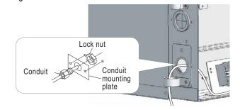
Figure 129: Exterior View of Conduit Installation.
