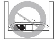
Do not terminate two wires on one side.
