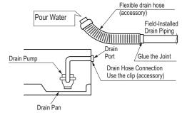
Figure 154: Checking the Drainage System.
