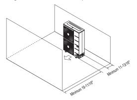
Where there are obstacles above, and on both suction and discharge sides (discharge side obstacle is higher than the outdoor unit).
