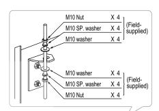
Install a canvas duct to the air outlet and air inlet so that vibration from the indoor unit does not carry to the duct or ceiling. Also, add insulation to the interior of the duct, and apply antivibration to the suspension bolts.
