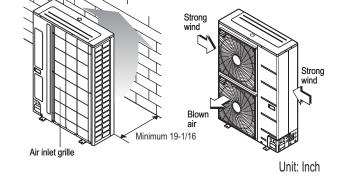
If the outdoor unit discharge side faces a wall, include a minimum of 19-11/16 inches between the outdoor unit and the wall. Install the outdoor unit so that the discharge port is set at a right angle to the wind direction.
