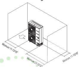
Obstacles above and on the air intake side. Obstacles above, on the air intake side, and on both left and right sides
