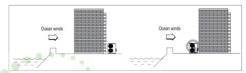
If the outdoor unit must be placed in a location where it would be subjected to direct ocean winds, install a concrete windbreaker strong enough to block any winds. Windbreaker height and width should be more than 150% of the outdoor unit, and be installed at least 27-1/2 inches away from the outdoor unit to allow for airflow.
