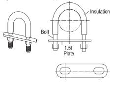
Figure 251: O-Ring Support with Insulation.
