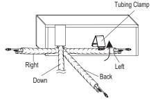
Figure 89: Piping Installed to the Left.
