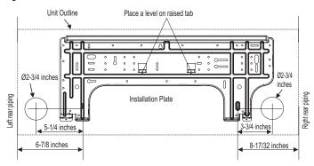
Figure 83: Installation Plate for LMN187HVT Units.
