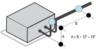
Figure 249: Pipe Support at Y-branch Fitting.
