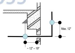
Figure 248: Pipe Support at Indoor Unit.
