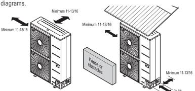
Ensure that the space at the back of the outdoor unit is a minimum of 11-13/16 inches, and include a minimum of 23-5/8 inches at the right side of the unit for service.
