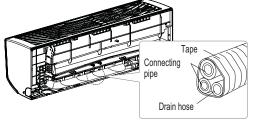
Figure 22: Piping Installed to the Right.
