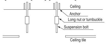
Figure 182: Installation Diagram.
