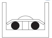
Terminate multiple power wires of the same gauge to both sides.
