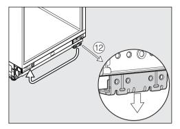
■ Take off lower retaining bracket <sup>12</sup> and replace it on the opposite side.
