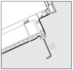
The feet can be adjusted with the spanner wrench supplied ③ or with an allen key ④.
