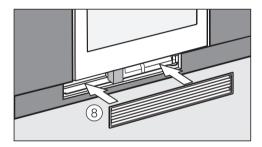
■ Fit ventilation grille ⑧ into the plinth facing. As you do this the foam block will be pushed back.
