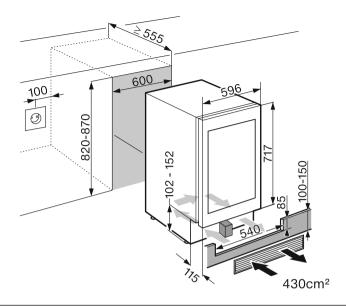
Before installation, ensure the building-in niche is the correct size. The specified ventilation cross-sections must be adhered to and the cut-out in the plinth facing must be aligned centrally with the appliance in order to ensure the correct functioning of the appliance.
