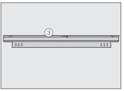
A bracket ③ is required to secure the filler panel, which is available from the Miele Spare Parts Department or from your dealer. The filler panel can be fitted above or below the appliance as required.
