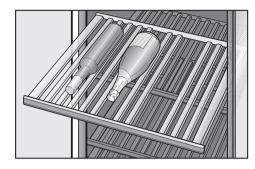
The three wooden shelves are on telescopic runners which can be pulled out to make it easier to store and remove bottles.
