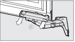
■ Remove screws ⑥ completely.
