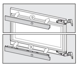
■ Clip covers ⑨ back on. Note the position of the notches on the hinges.
