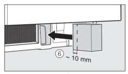
■ Insert foam block ⑥ supplied into the appliance plinth.
