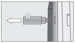
Deactivate the door opening mechanism by pulling out the door opener.
