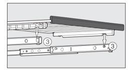
■ To replace the shelf, click it into place on the extended runners ③. The notches on the wooden shelf fit into the retaining brackets. The magnetic strip should be pointing forwards.
