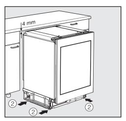
■ Screw adjusting feet ② to 4 mm less than the height of the niche.
