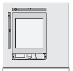
Align the appliance horizontally and vertically. If it is not level the appliance can distort.
