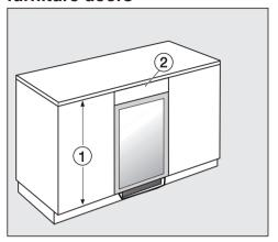
If adjacent furniture housing doors ① are taller than the wine conditioning unit door, the wine conditioning unit can be aligned to the unit doors using a filler panel ②.
