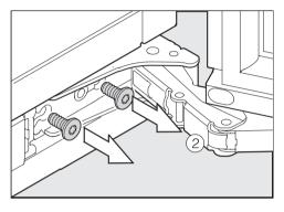
■ Remove screws ② first from the lower hinge.
