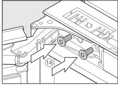
■ Tighten the screws in upper hinge <sup>14</sup>.
