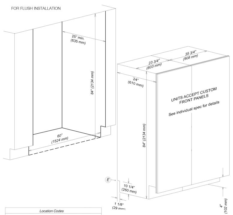
E- power cord for refrigeration unit- 5 foot- NEMA 5-15 molded plug power supply connects lower left rear of units
