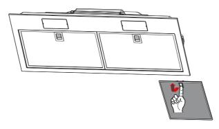
• Remove the bottom of the Range Hood by 4 screws **12b** as shown.
