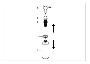
Install dispenser base (b) with washer (c) attached into the hole in the countertop. Re-install mounting nut (d) on the dispenser base (b) from underneath the countertop. Tighten mounting nut (d) by hand
