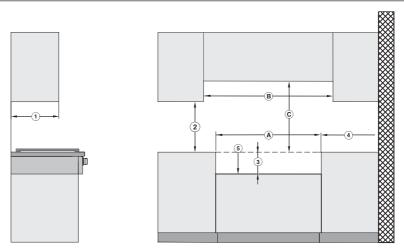
® In case of combustible construction, an additional minimum clearance of 6" (150 mm) on each side is necessary. Ensure local codes are observed.
