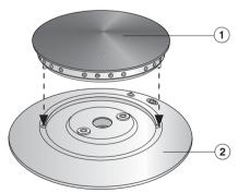
■ Place the burner cap, ①, onto the burner base, ②, so that the notches fit into the holes (see arrows).
