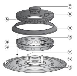
■ Place burner head ⑩ on to burner base ⑪ so that the thermocouple ⑪ and the ignitor ⑫ extend through their respective holes in the burner head.
