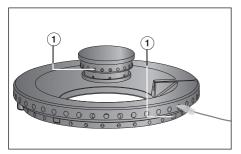
■ Clean any soiling from the flame openings ① with the brush supplied.
