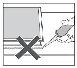
The cooktop must not be permanently sealed into the countertop when installed. The sealing strip under the edge of the cooktop provides a sufficient enough seal.
