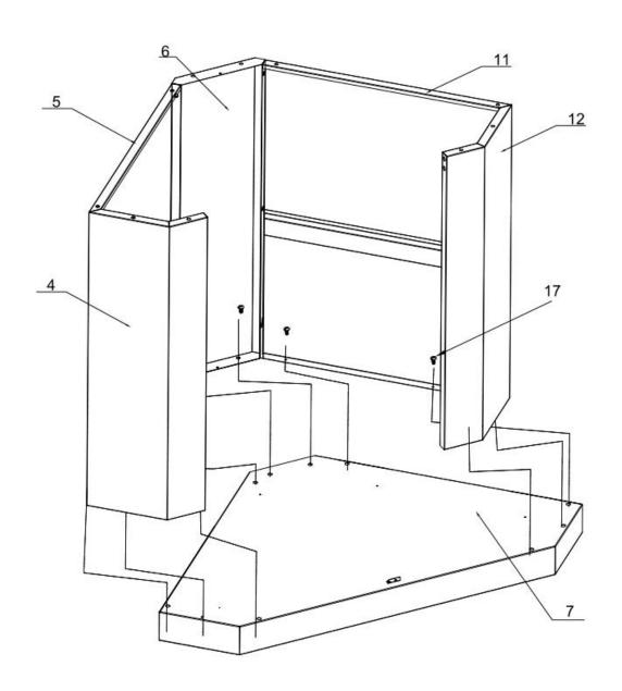
1. Use 4 pcs Part # 17 to connect Beam welding assembly (Part # 14) to Part # 4 and Part # 12. Do not over-tighten all the screws until parts are lined up.
